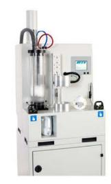
Penetration, filter resistance and flow rate data are transferred in near real time via USB cable to a nearby connected laptop running data acquisition program recording values and producing charted plots of resistance and penetration.
