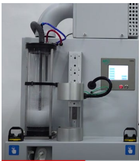
ATI 100Xs Automated Filter Tester with chuck open
