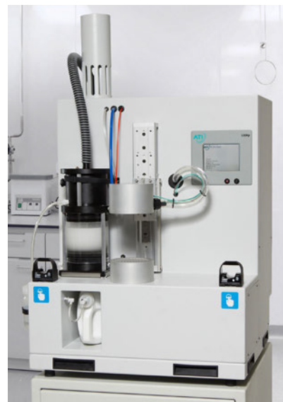
Salt Aerosol Automated Filter Tester - ATI 100Xs
