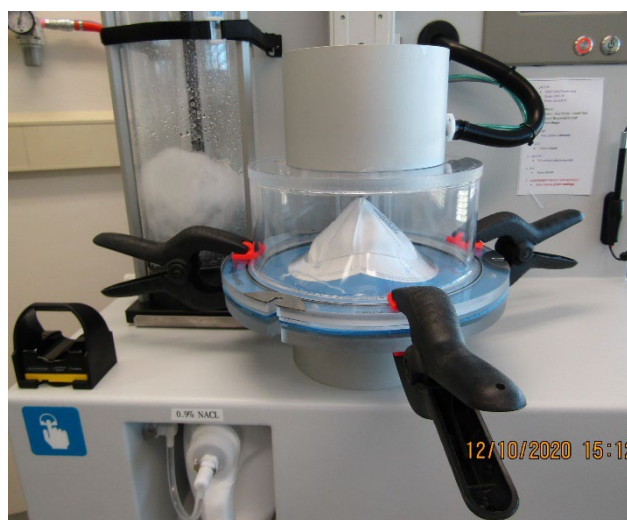
Close up of respirator & an adapter in the closed chuck
