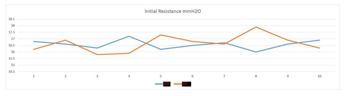
FINDINGS: Penetration - for these samples both operators recorded identicle penetration average (0.64%) with a SD of 0.001 % (type A uncertainty) indicating very good reproducability. The instrument accuracy specification for penetration is +/- 1% of reading. Initial Resistance -The standard deviation of means between operators was 0.057 mmH2O. the instrumen accuracy specification for resistance is +/- 0.625 mmH2O
