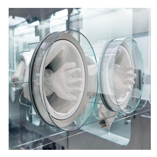
4.21 The materials used for glove systems (for both isolators and RABS) should be demonstrated to have appropriate mechanical and chemical resistance. The frequency of glove replacement should be defined within the CCS.
