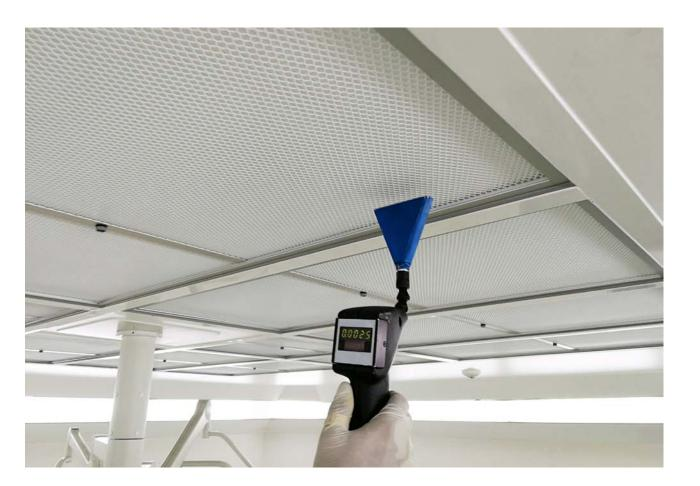
4.27 For cleanroom classification, the total of particles equal to or greater than 0.5 and 5 μm should be measured.
