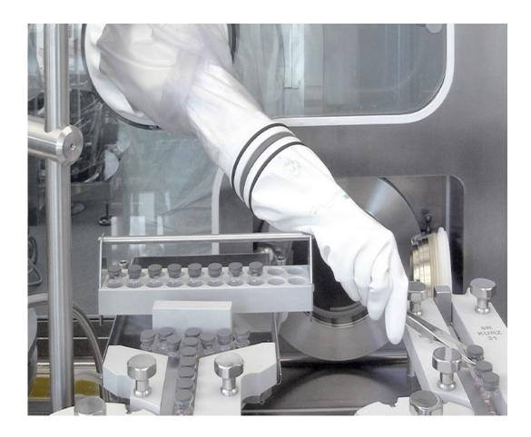
4.4 Grade A: The critical zone for high-risk operations (e.g. aseptic processing line, filling zone, stopper bowl, open primary packaging or for making aseptic connections under the protection of first air)...
