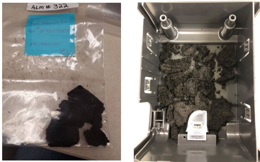
Figure 2. (L) Return 307803629 is IN461S device with Serial Number P1165312101A5 built June 5, 2014 per the eDHR. (R) Representative PE-PUR foam degradation utilized for the biological endpoint studies.
